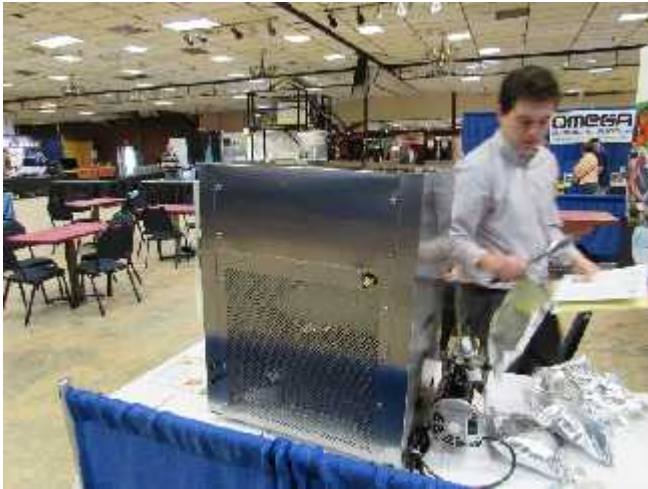
Side view of the Harvestright™ freeze-drying machine. Not the complex compressor, vacuum and refrigeration equipment at the rear,
