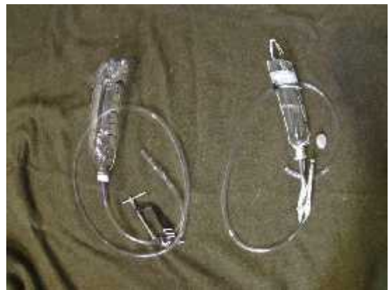
C-clamp flow control on the left and a vice-grip pliers used on the right. The small vice-grips worked well because the adjustment knob permits easy flow adjustment.
