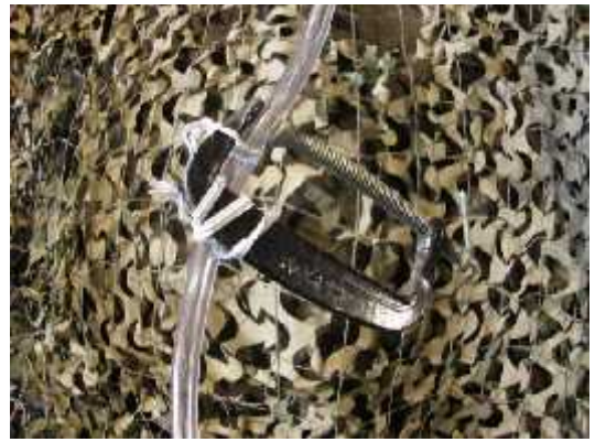
Detail of C-clamp flow control method
