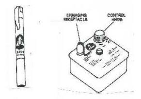
Dosimeters are intended to be worn in the pocket and checked frequently to determine how much radiation the wearer has been exposed to. They come with a charger and instructions. A charger and two dosimeters sell for about \$40.00
